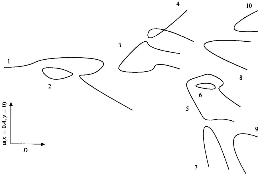
FIGURE 15. Schematic diagram showing decoupling in square ducts resulting from addition of stickiness.
